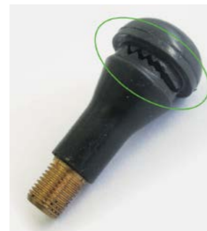
Old, torn valve
