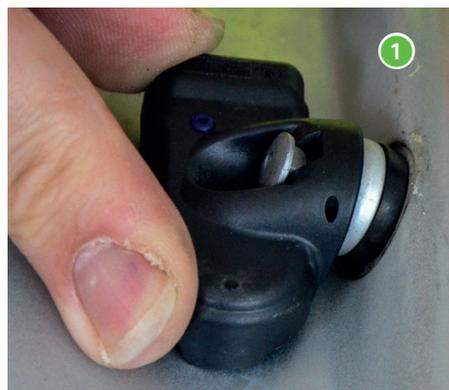
If all the adjustable angle space is not used, it may cause the grommet not to lie correctly on the rim which can lead to leaks. 2
