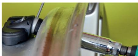
The cross-bore in the base of the valve is for disassembly. The disassembly pin can be used to loosen a stuck hexagonal nut.
