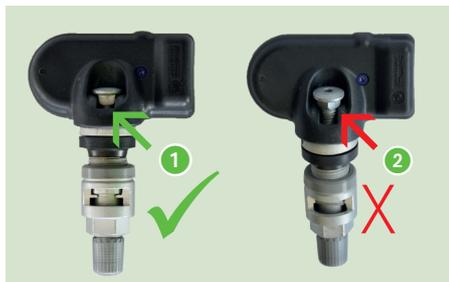
The screw must be pre-tightened sufficiently so that it can not turn when the valve is rotated in the housing.
