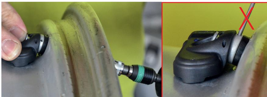
The torque of the bolt is created by the breaking properties of the special shear-collar in hex-nut, which means you must not use the pin during assembly! The valve must turn until the bolt is tightened.
