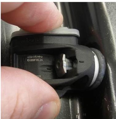
If all the adjustable angle space is not used, it may cause the grommet not to lie correctly on the rim which can lead to leaks.
