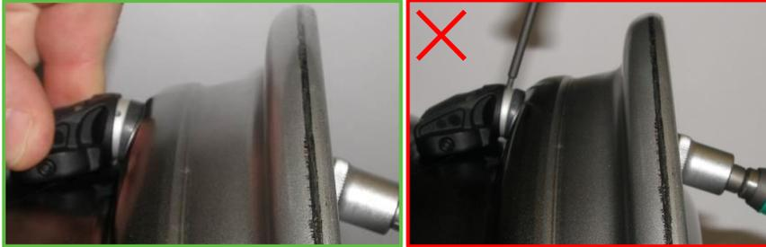
The torque of the bolt is created by the breaking properties of the special shear-collar in hex-nut, which means you must not use the pin during assembly! The valve must turn until the bolt is tightened.
