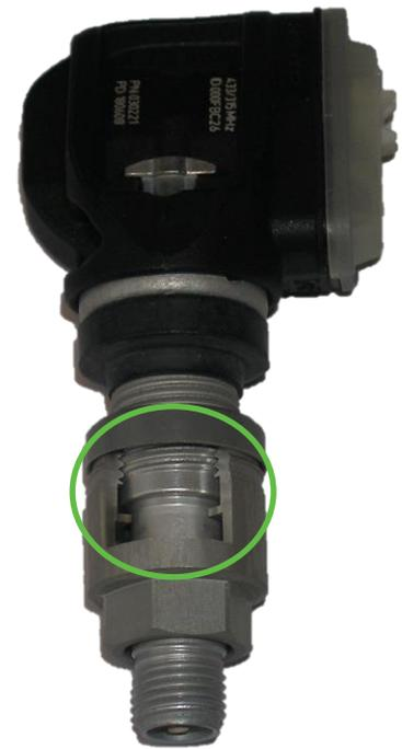
The shear-collar breaks at less than 3.5 Nm
