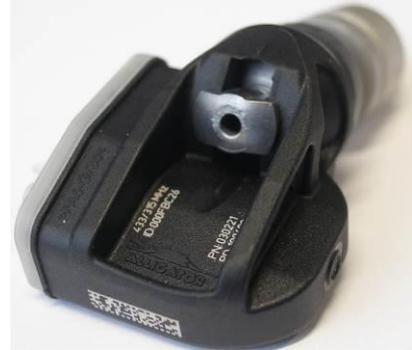
**The square section at the base of the screw must be properly seated in the slot.**
