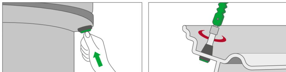
Press the valve in by hand without using too much force. Or mount gently with the ALLIGATOR standard valve mounting tool. The valve must be pulled in axially to the rim hole – do not tilt.
