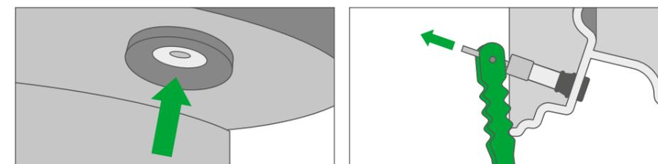
Now the valve can simply be pulled outwards through the valve hole with the ALLIGATOR standard valve mounting tool.
