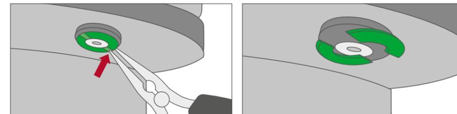
To disassemble, use tongues or a screwdriver to crack the patented thrust washer at the marked predetermined breaking point and remove.
