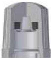
Cross-section valve cap with built-in seal.
