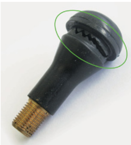
Old, torn valve
