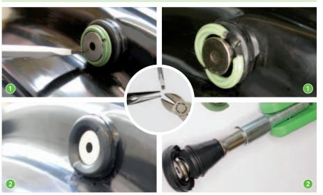
2 Now the valve can be simply pulled out through the valve hole, using the ALLIGATOR standard mounting tool.
